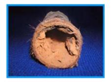
Indications that galvanized steel water pipe is approaching or at the end of its service life are: pinhole leaks or corrosion on the exterior surface of the pipe where pinhole leaks have temporarily self-sealed from mineral accretion/build-up, reduction in water flow, and/or the regular discharge of rusty colored water each time a tap is opened.
